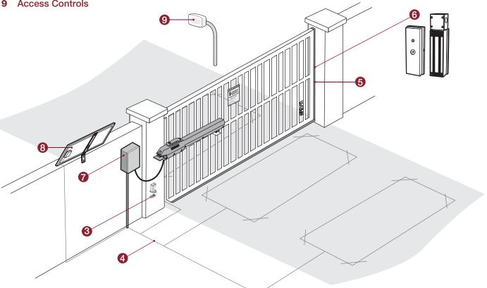
LiftMaster gate operators comply with UL 325 standards. Important: To be compliant with UL 325 and industry safety guidelines, gualified monitored external entrapment protection devices such as photoelectric sensors or edge sensors are required to be installed with this operator
